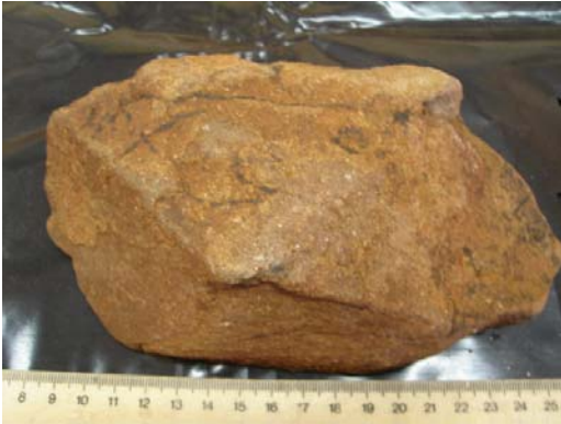
Fig. A1.1.11 Sandstone. \rho_d = 2\,858 \text{ kg m}^{-3} .
