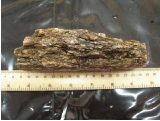
Fig. A1.1.4 Mylonite-gneiss. \rho_d = 2\,560\text{ kg m}^{-3} .
