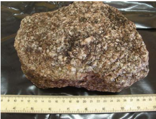
Fig. A1.1.1 Coarse-grained porphyritic granite. \rho_d = 2537 \text{ kg m}^{-3} .
