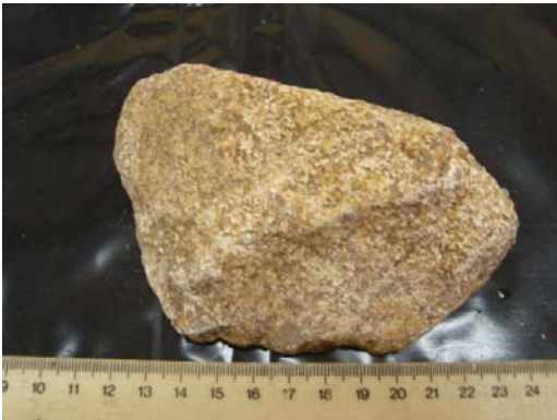
Fig. A1.1.2 Medium-grained granodiorite. \rho_d = 2609 \text{ kg m}^{-3} .
