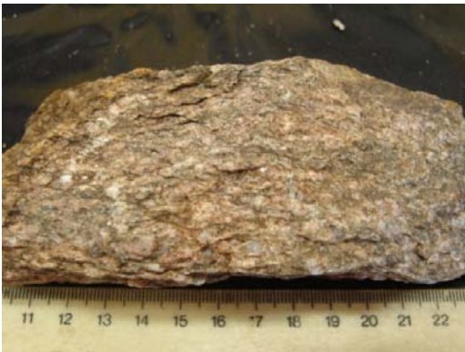
Fig. A1.1.3 Augen-gneiss. \rho_d = 2594 \text{ kg m}^{-3} .
