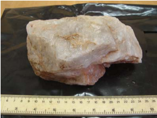
Fig. A1.1.5 White quartz. \rho_d = 2\,634\text{ kg m}^{-3} .
