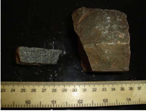
Fig. A1.1.10 Quartz-diorite/gabbro (left), \rho_d = 2\,995 \text{ kg m}^{-3} ; basalt (epidiorite) (right), \rho_d = 2\,825 \text{ kg m}^{-3} .
