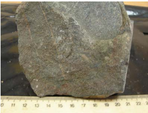
Fig. A1.1.6 Metabasaltic greenstone. \rho_d = 2\,982\text{ kg m}^{-3} .
