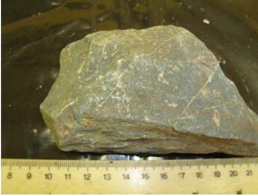
Fig. A1.1.7 Amygdaloidal metabasaltic greenstone. \rho_d = 2\,976 \text{ kg m}^{-3} .
