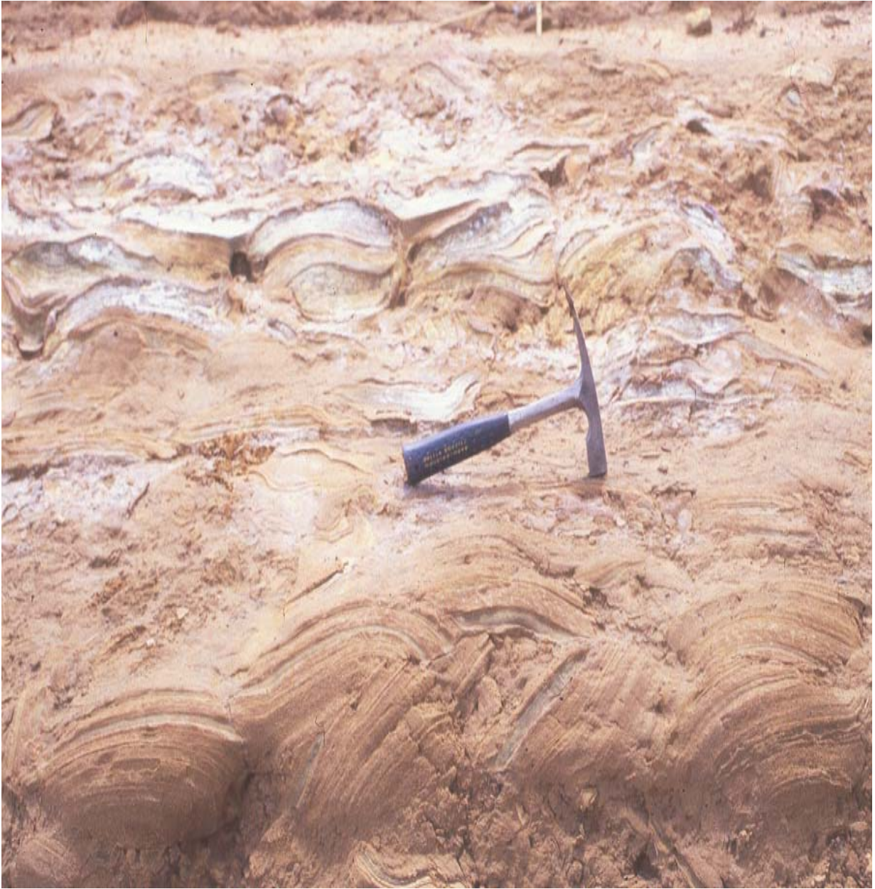
Figure 2.8. Compacted surface crust on the slimes dump at Athens lowers percolation of water and forms a hard pan on the sides of the dump. The reduction of percolation results in water logging on top of the slimes.
