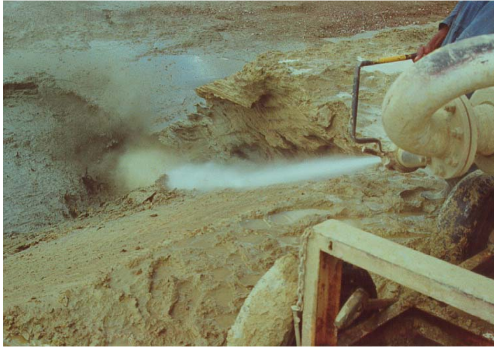
Fig 1.2 Slimes being mined hydraulically and flowing to the processing tanks
