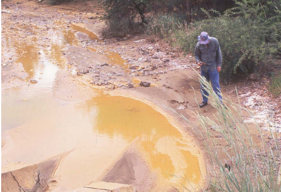
Figure 3.1 Yellow boy, typical indicator of AMD in a stream adjacent to the Falcon shaft at Athens Mine.
