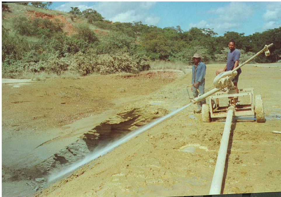
Figure 1.1. Re-working on the Falcon old dump. Mining is done using water under pressure to break the compacted slimes. The mining process is affecting the surrounding vegetation and the nearby stream.
