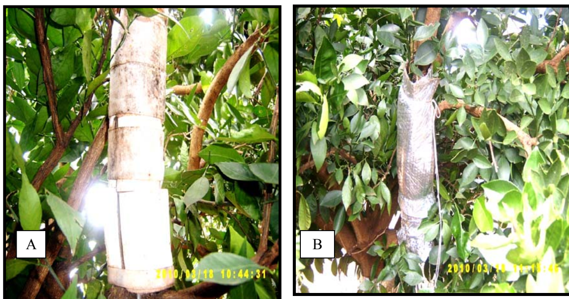
Figure 3.6: An illustration of the installation of the SGB 35-ws gauge on the branch of a tree a) before and b) after wrapping with an aluminised shield.
