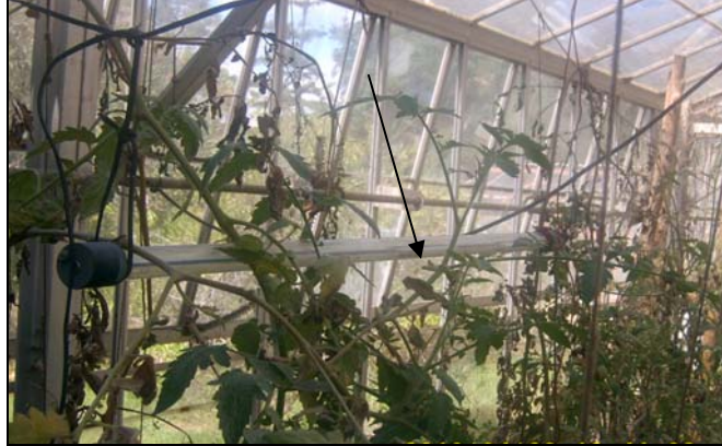
Figure 3.3: A suspended tube solarimeter in the greenhouse
