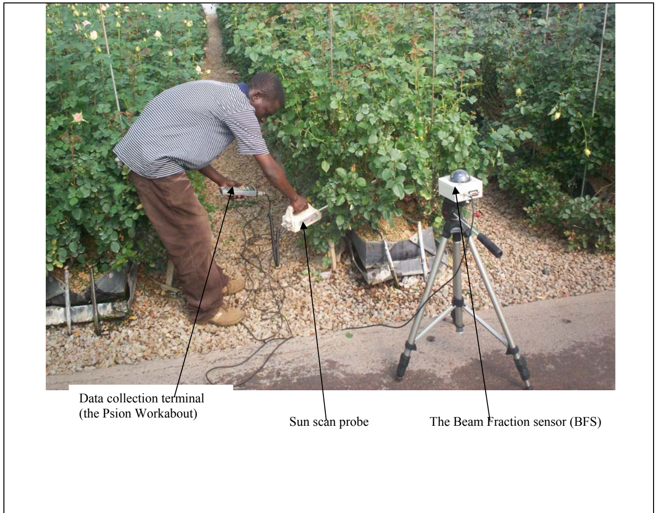
Figure 3.7: Determination of LAI using a sun scan canopy analysis system [ref: personal digital camera]
