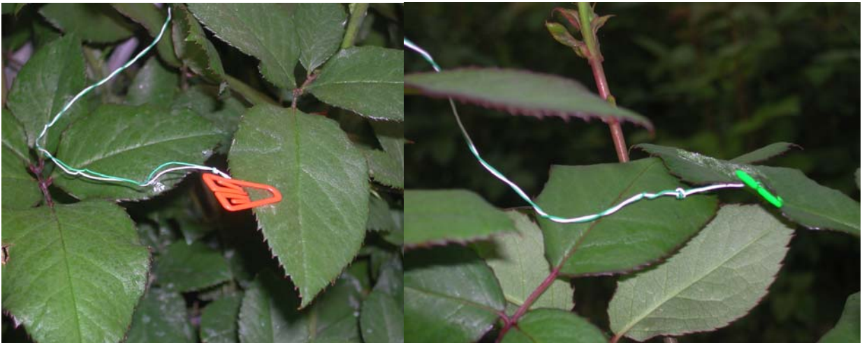
Figure 3: 9: Attachment of the thermocouples on the underside of leaves in the greenhouse
