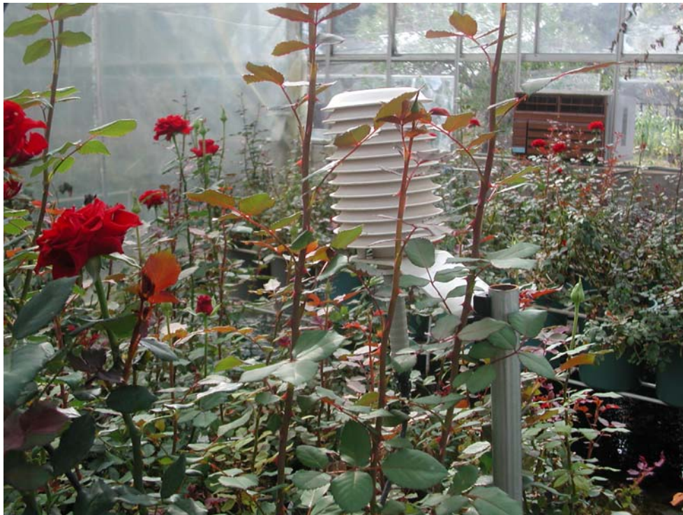
Figure 3: 8: The probes used to measure the greenhouse air temperature and humidity in the experimental greenhouse, Biological Sciences Department, UZ.
