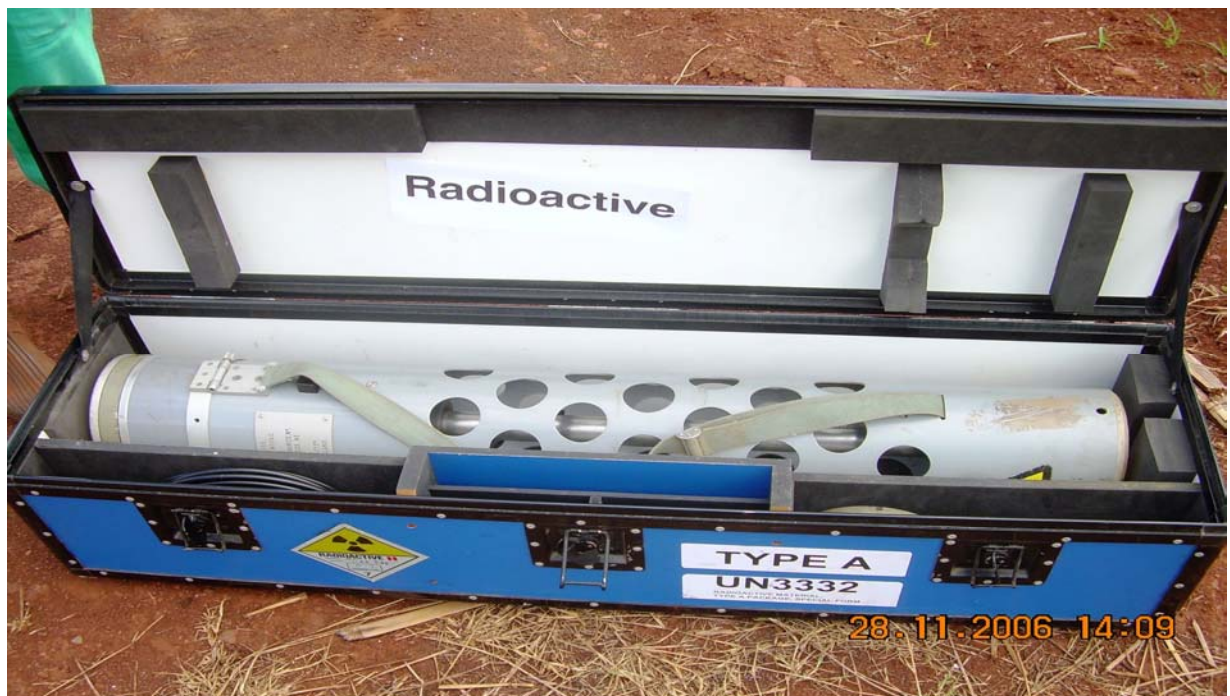
Figure 3. 4 The Wallingford neutron probe used for soil moisture measurement
