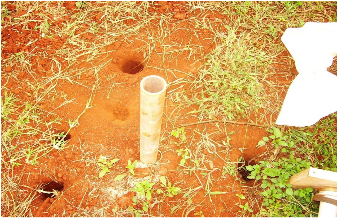
Figure 3.5 Collection of soil samples around the access tube for neutron probe calibration.
