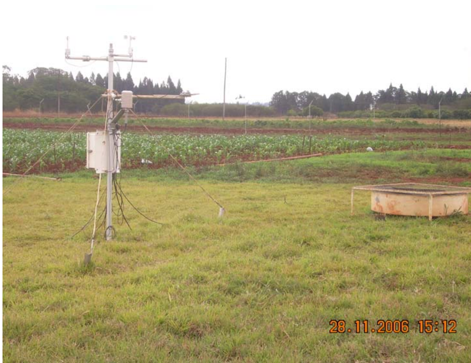
Figure 3.3 The automatic weather station used to collect daily weather data for the computation of the FAO Penmen -Monteith equation.
