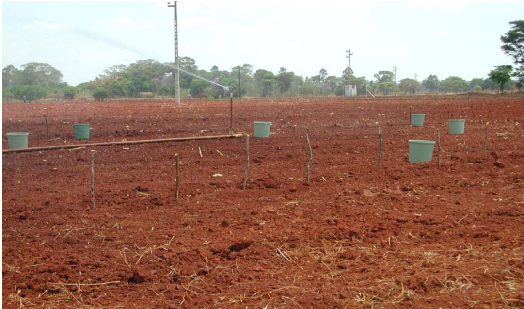
Figure 3. 2 The determination of the application rate using catch can method
