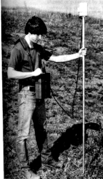
Fig. 3.9 Portable proton precession magnetometer (Dobrin and Savit, 1988). The sensor is mounted on an aluminium pole of about 2 m long.
