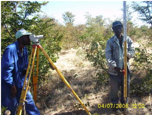
Fig. 2.5 The 'dumpy level' and staff with a vertical level spirit bubble. A Sokkisha B2 A77744 dumpy level was used.
