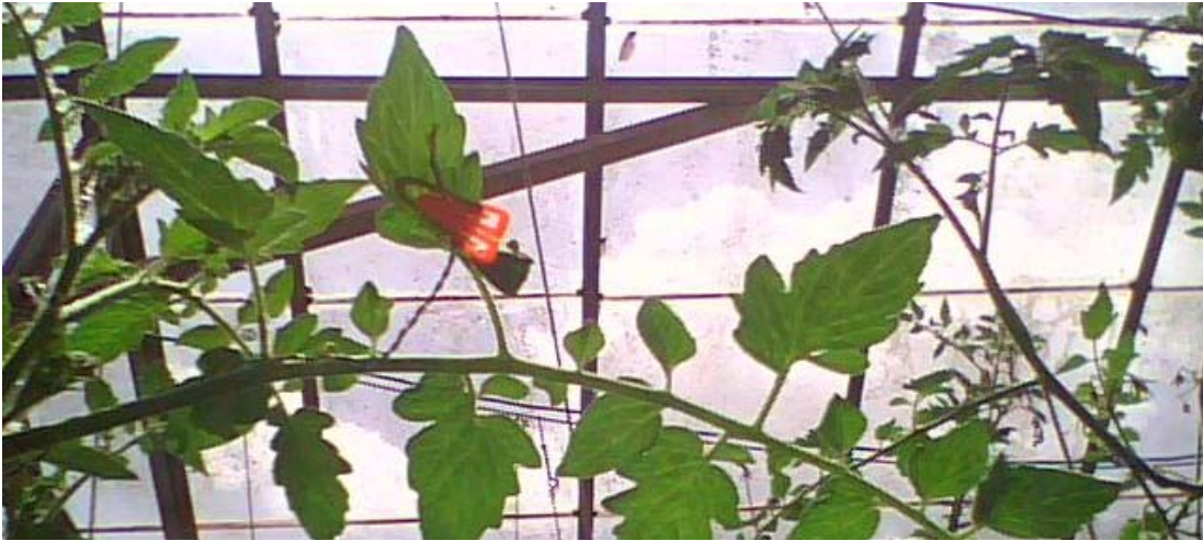
Figure 3.12: A thermocouple clipped onto the underside of a leaf so as to measure leaf temperature.
