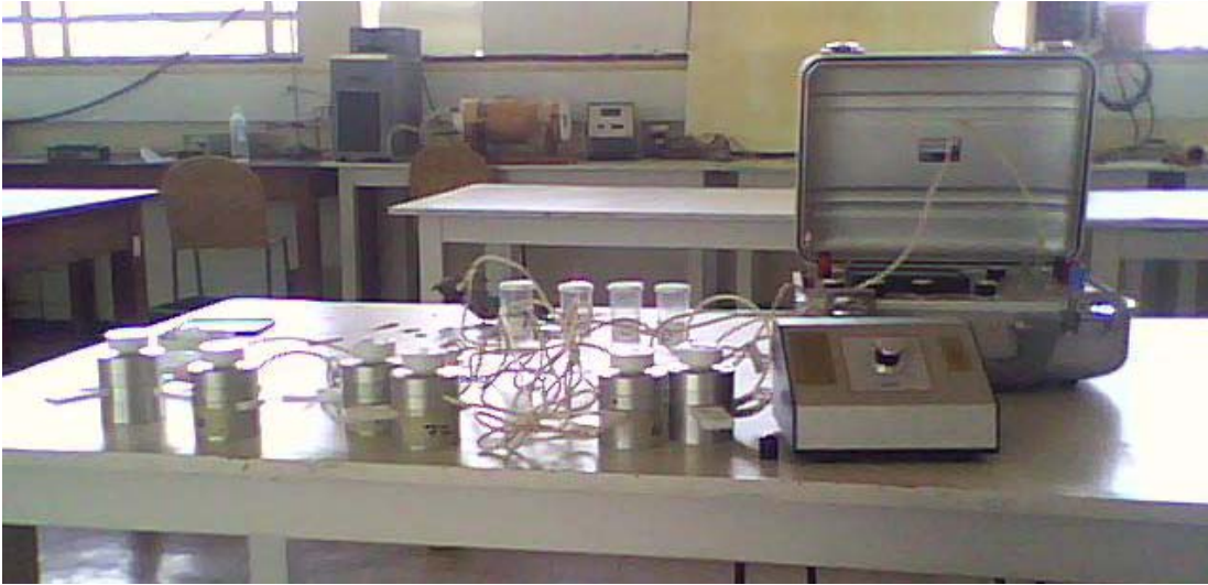
Figure 3.10: The Wescor Thermocouple Psychrometer kit with sample chambers, switchbox, microvoltmeter and the four airtight plastic chambers that were used to collect the samples.
