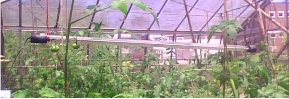
Figure 3.5: A tube solarimeter measuring radiation above the canopy of the tomato crop
