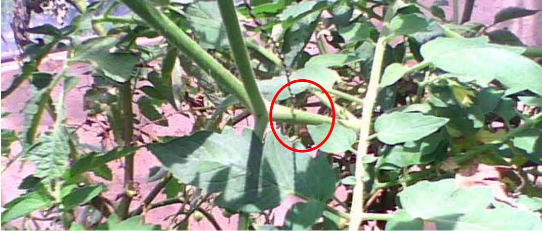
Figure 3.13: A thermocouple inserted into a stem (circled in red) to measure stem temperature.
