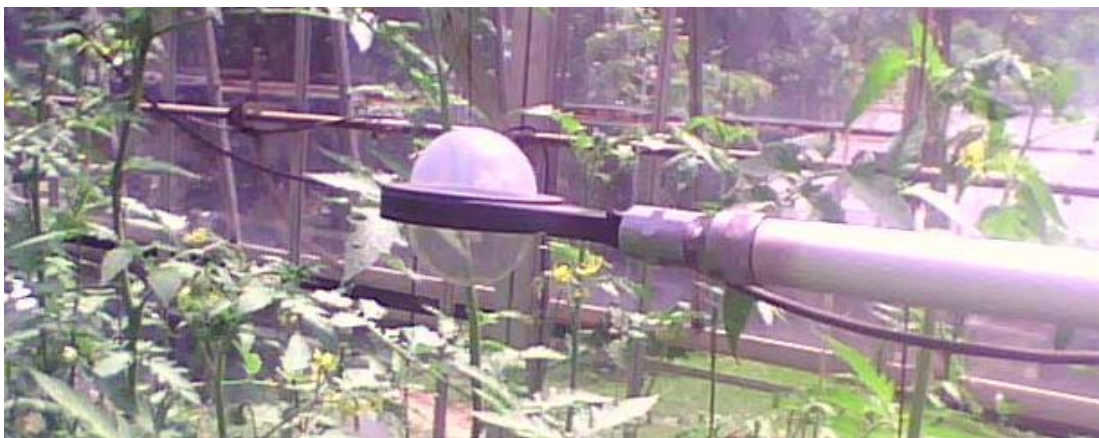
Figure 3.7: The Q7.1 net radiometer (REBS, Washington, USA) used in the greenhouse
