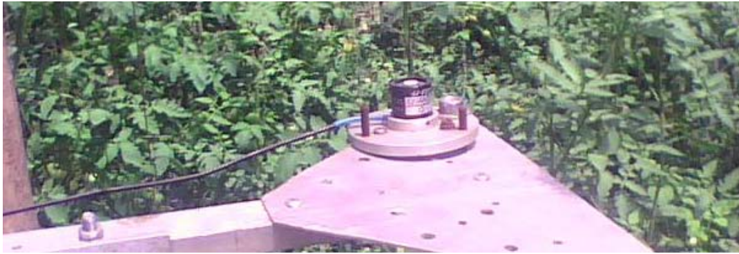
Figure 3.8: The LI-190SZ Quantum Sensor (LI-COR Inc, Nebraska, USA) used in the greenhouse
