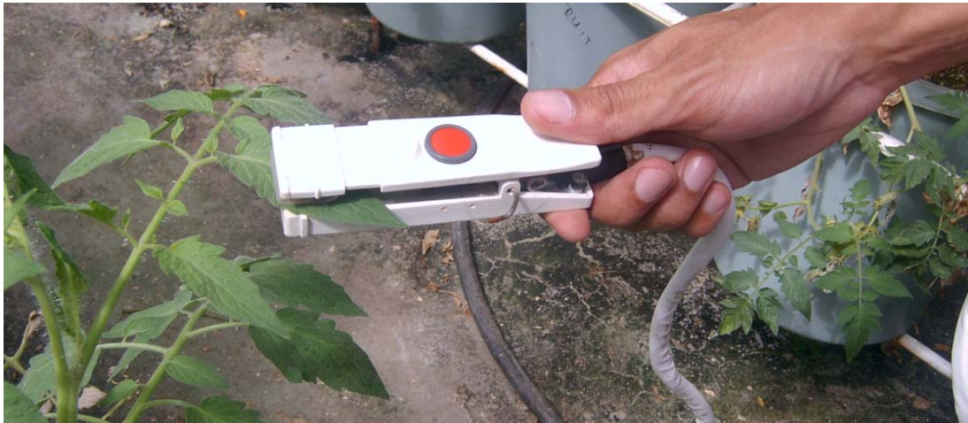
Figure 3.11: The measurement of stomatal resistance of the leaves of tomato plants using the AP4 porometer (Delta-T Devices, Cambridge, UK)
