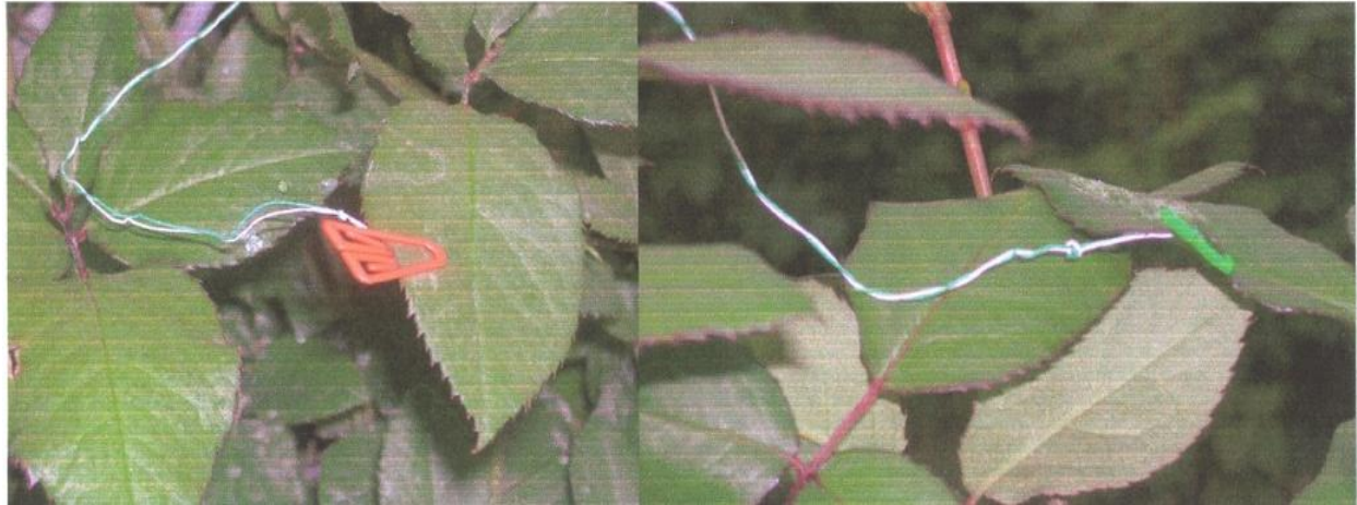
Figure 3. 5: The picture showing thermocouples attached to the underside of the leaf for measuring leaf temperature
