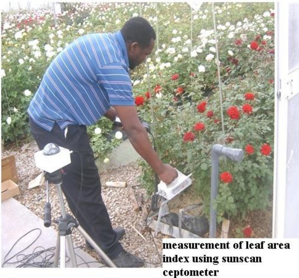
Figure 3. 9: Showing the set up for the sunscan ceptometer for measuring the leaf area index.
