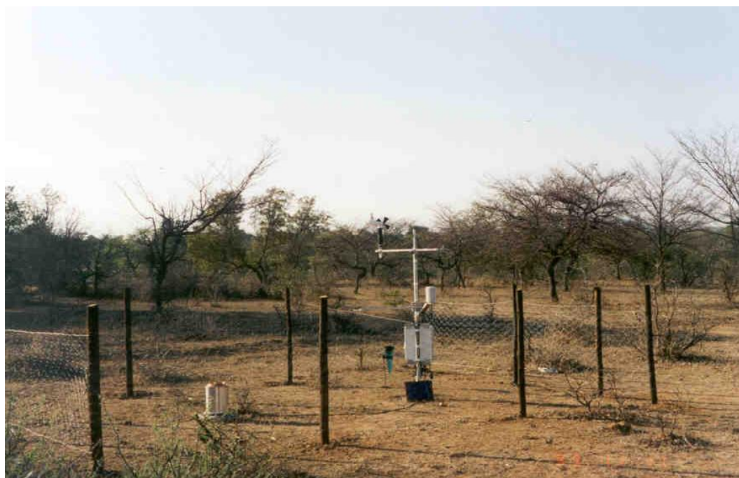
Figure 5.2: The automatic weather station at Mutangi catchment.
