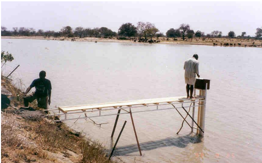
Figure 5.4: A view of the digital water level recorder (in the box) at Mutangi dam.
