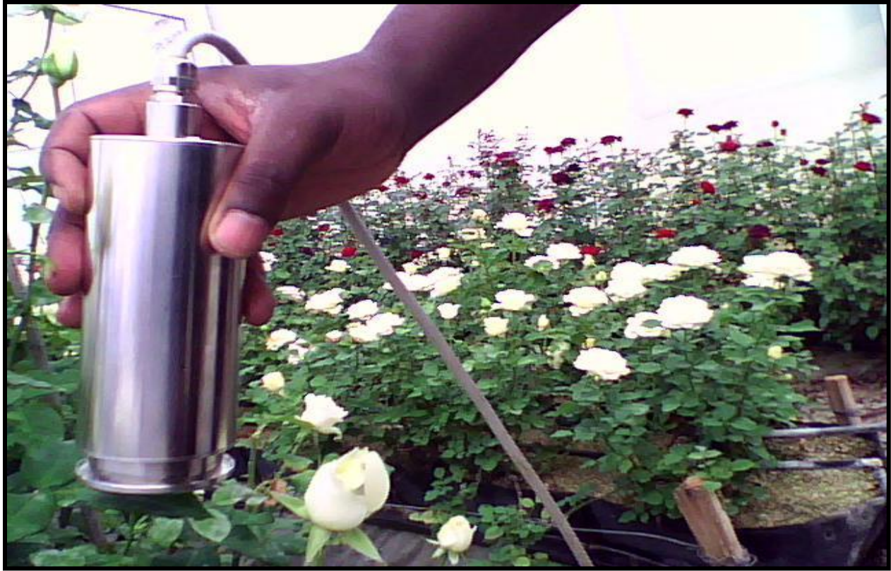
Fig 3.10: Leaf temperature measurement taken by a radiation thermometer
