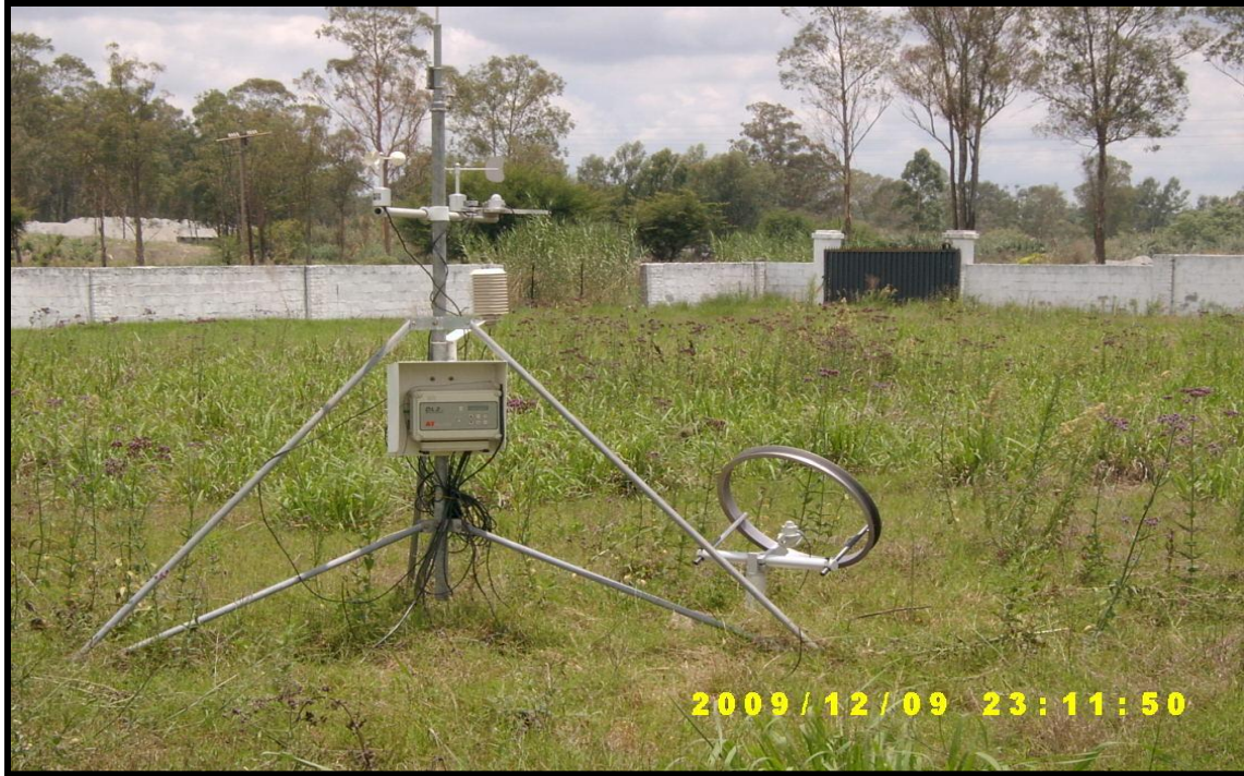
Fig 3.6: The outside Automatic Weather Station (AWS) at Floraline (Pvt) Ltd, mounted with all sensors and the shade ring for measurement of diffuse radiation.
