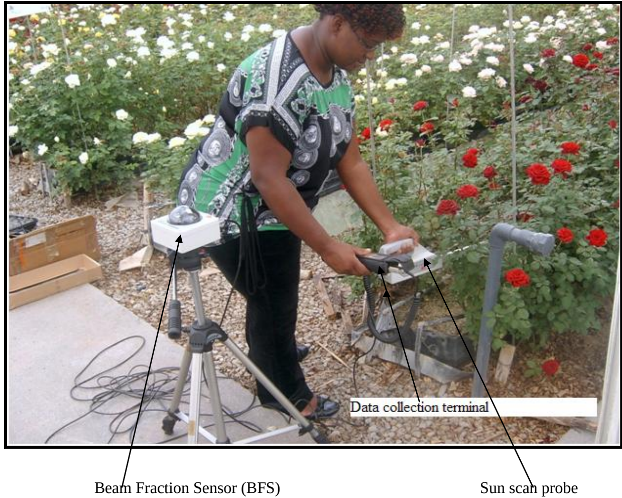
Fig 3.8: Estimation of the Leaf Area Index (LAI) using a sunscan canopy analysis system
