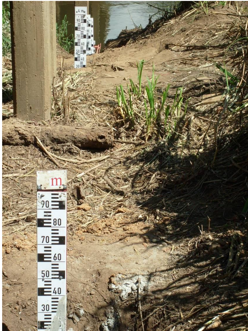
Figure 3.4 River Gauging Station in the Mkindo River
