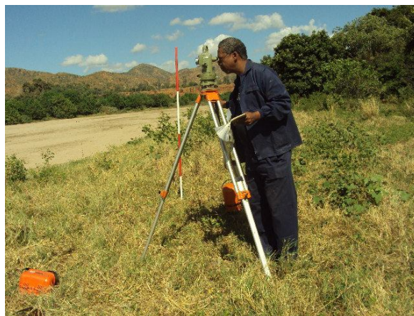
Figure 3. 10: Measuring the reduced levels as well as the distance using a Theodolite
