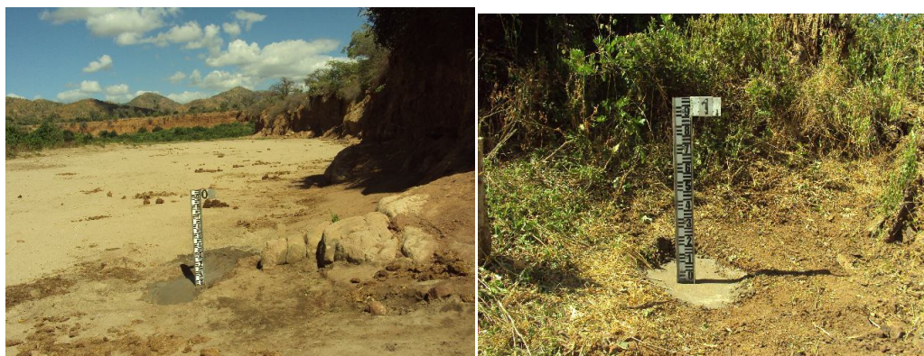
Figure 3. 11: Installed gauging plates and the presence of rock materials at Rukomechi gauging station
