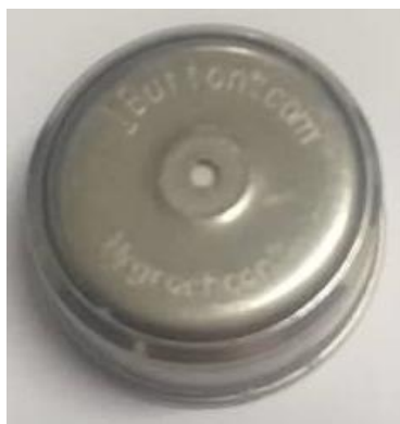
Figure 6.1: The thermocron i-Button used for recording temperature and RH inside the two climate chambers, and the ambient temperature and RH (outside the chambers), and inside the tested storage facilities (Source: Charles Singano, the Department of Agricultural Research Services, Lilongwe, Malawi).
