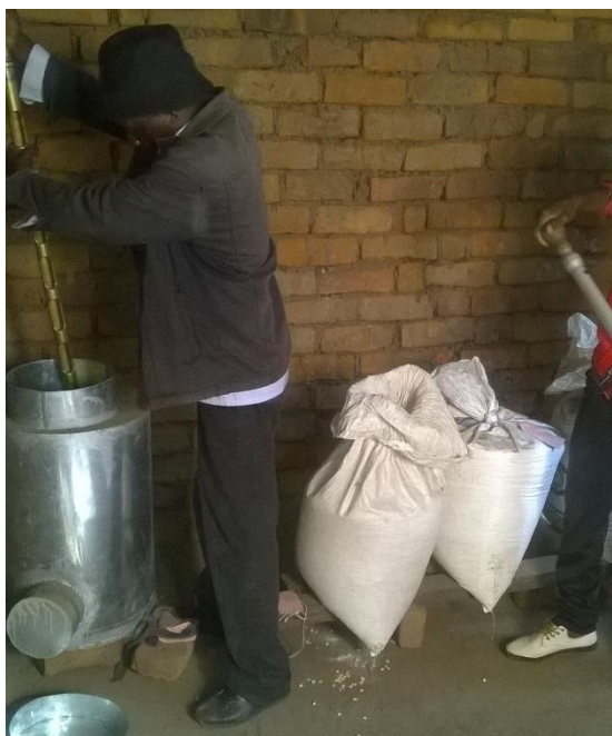
Figure 5.2: Sampling maize grain in a metal silo using a multi-compartmented sampling spear (Source: Charles Singano, the Department of Agricultural Research Services, Lilongwe, Malawi).
