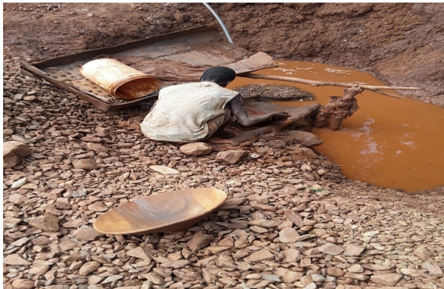
Plate 7: Temporary water pond for gold processing. Source: M. Jomboro, 2018.
