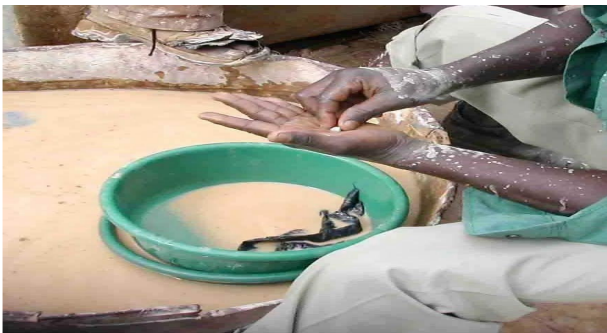
Figure 4. Hand mixing of gold concentrate with mercury for amalgamation.
