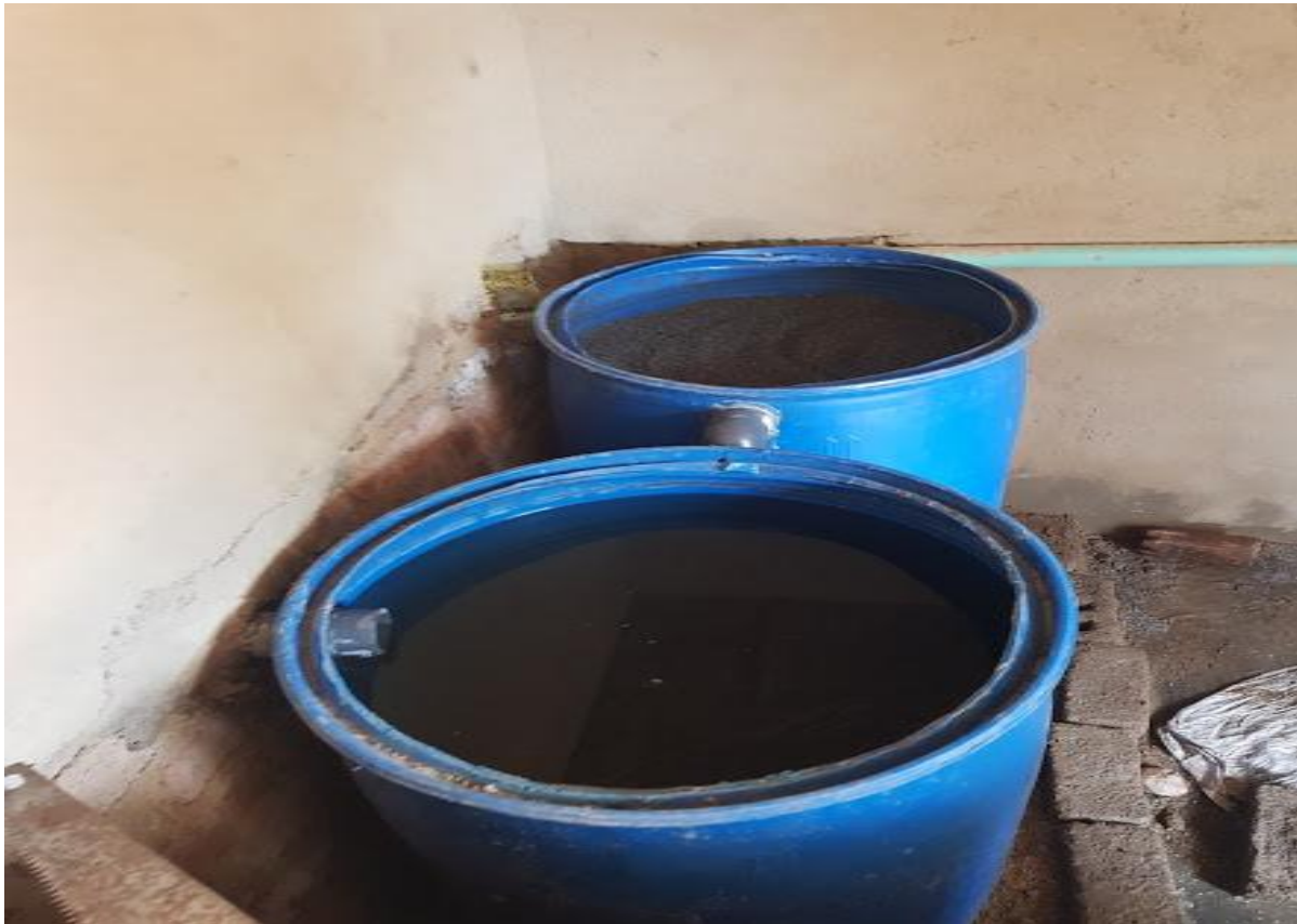
Figure 6. Adsorption circuit consisting of drums loaded with activated carbon and pregnant leach solution.
