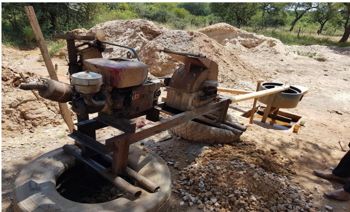
Figure 3. Setup of a typical diesel-powered hammer mill connected to a gravity concentrator for ASGM operations.
