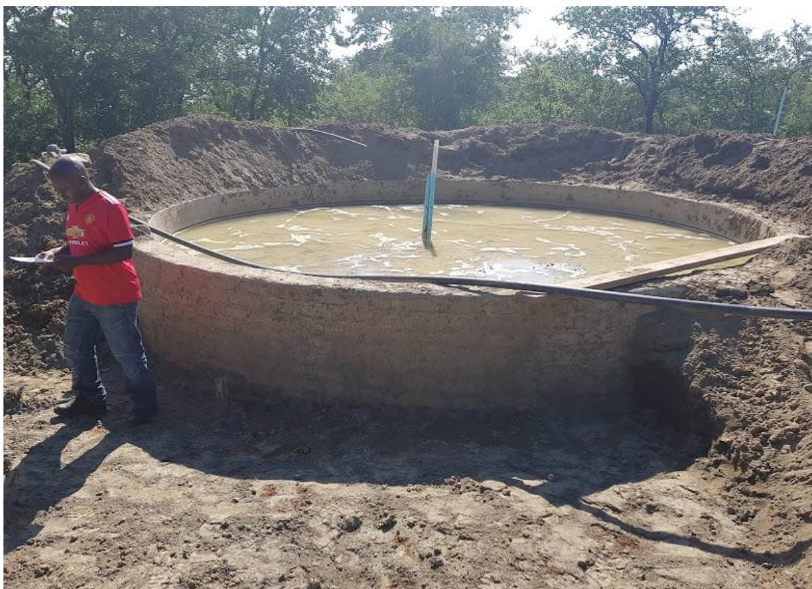
Figure 5. Vat leach tank for gold recovery from tailings in ASGM operations.
