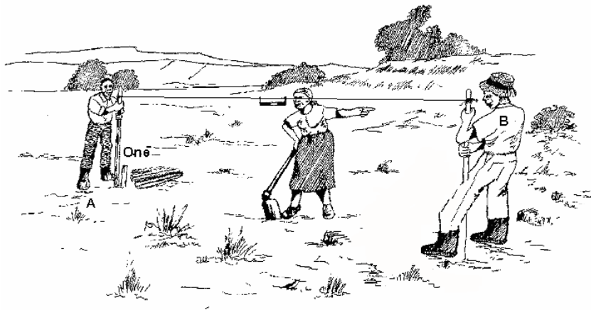
Figure 25 Step 2 - line level
