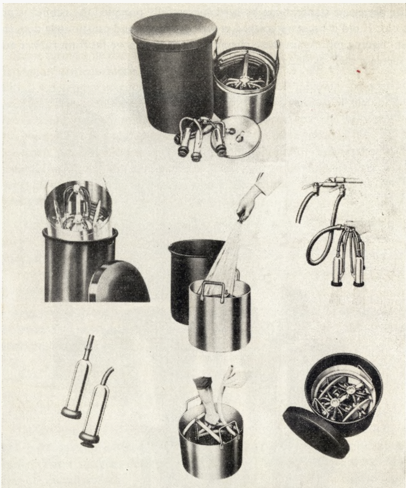
PLATE 6. The immersion system of cleaning milking equipment.
