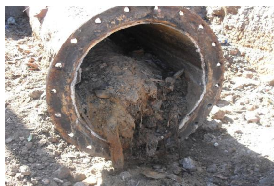
Figure 4.11 Poor workmanship in sewer connections can cause silt to enter and block sewerage network systems
