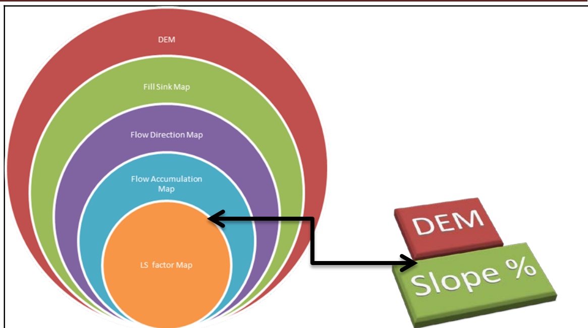
Figure 10: Schematic procedure to produce LS factor Map
