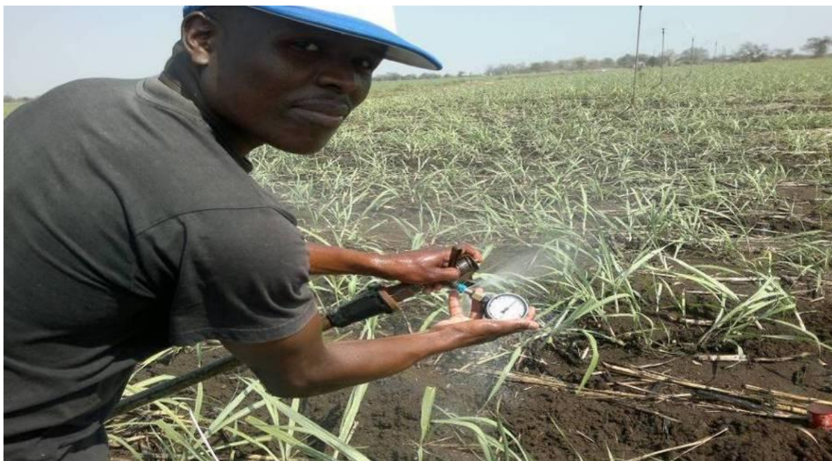
Figure 4.1: Pressure measurement using a pitot tube end pressure gauge at Ziyanhle FA
