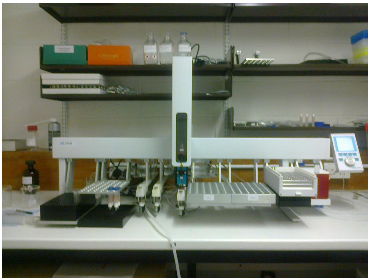
Figure 2: The CTC-PAL the Ultra High Throughput System (CTC Analytics AG, Zwingen Switzerland)
