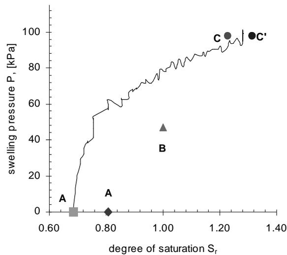
Figure 5.3 Mobilisation of swelling pressure with increase in degree of soil saturation
