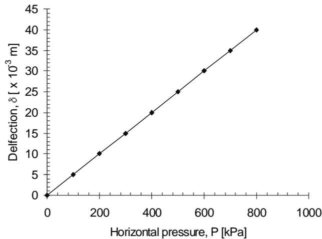
Figure 3.2 Membrane deflection with increase in horizontal pressure
