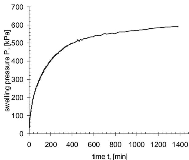
Figure 5.5 Mobilisation of swelling pressure along flooding path
