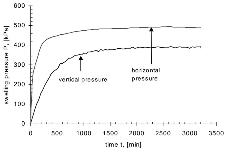
Figure 6.1 Mobilised swelling pressure for a horizontally sampled sample
