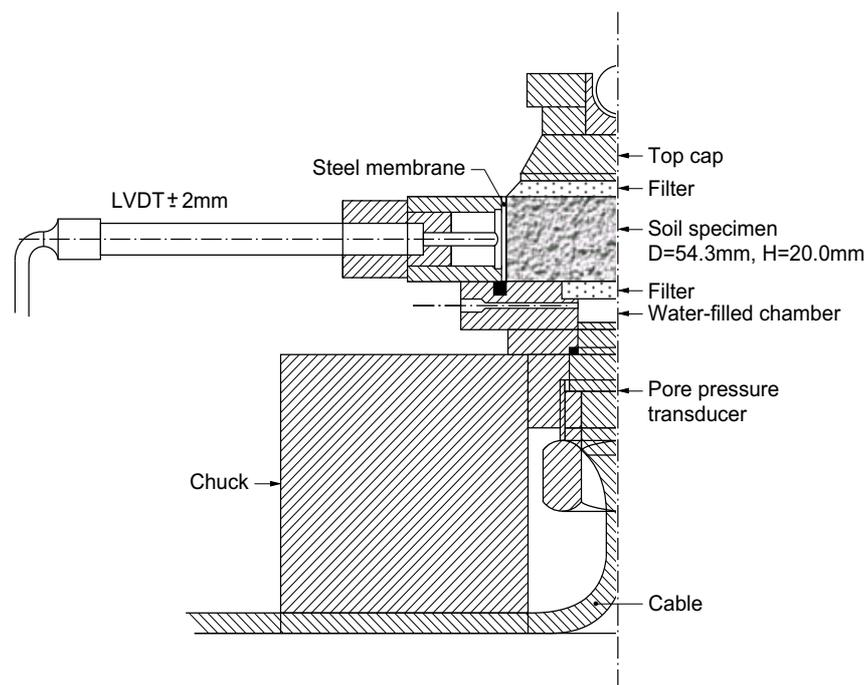
Figure 3.1 (a) Simplified cross-section of the split-ring oedometer (after Senneset, 1989)
