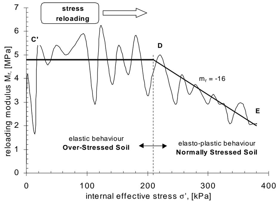
Figure 7.6 Reloading tangent modulus plot
