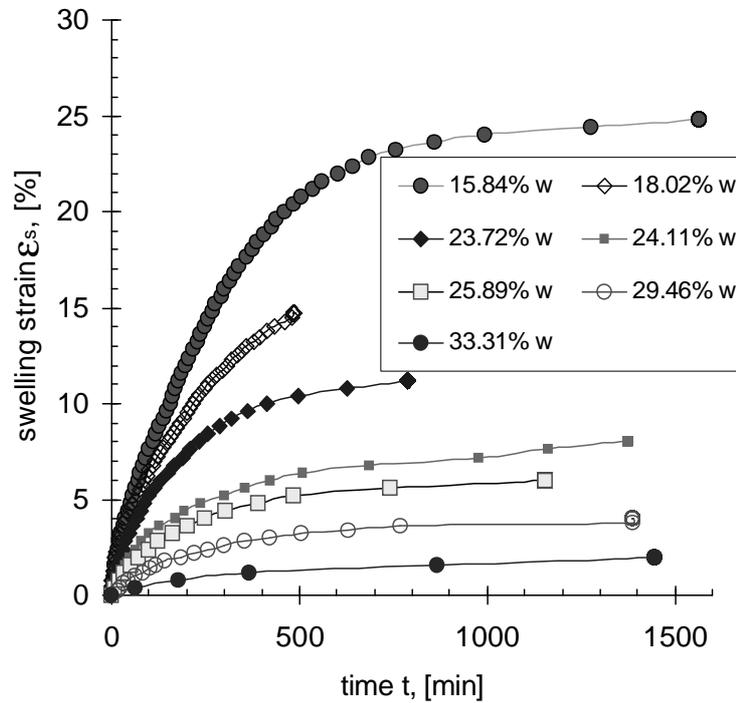
Figure 4.10 Time-swelling strain plot for a range of initial water content
