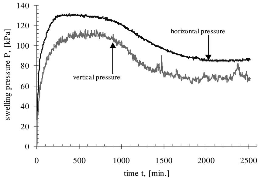
Figure 4.2 Mobilisation of swelling pressure with time (pressure-gradient)
