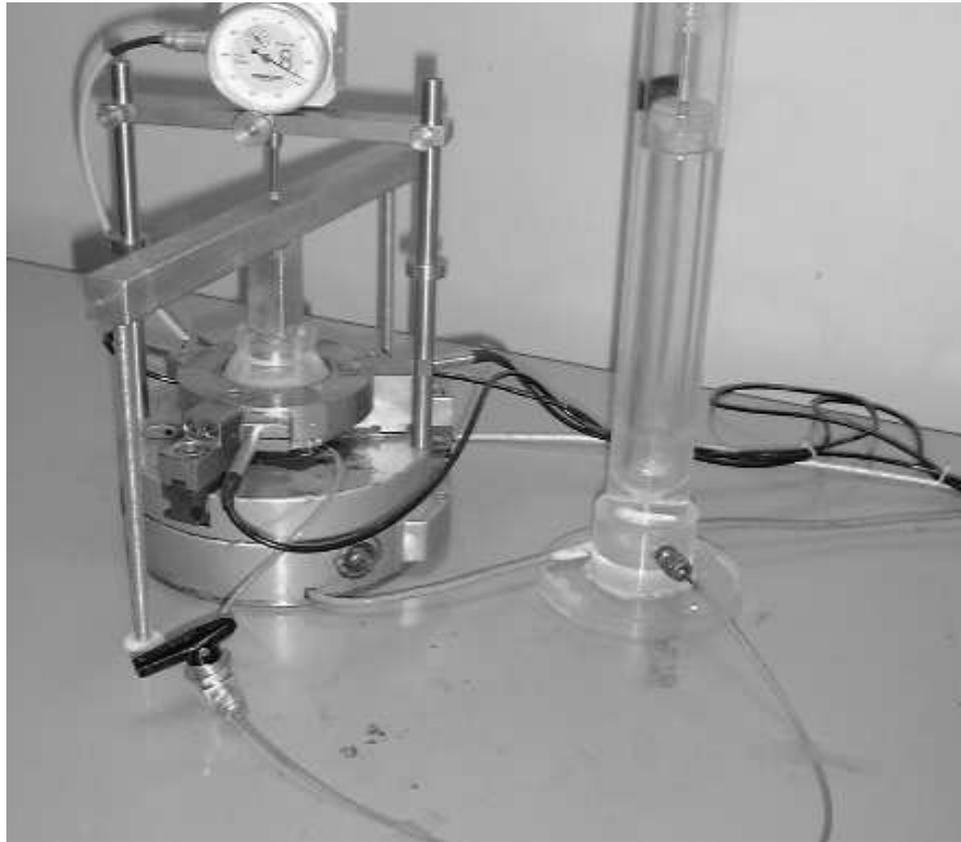
Figure 3.7 Oedometer set up for free swelling tests
