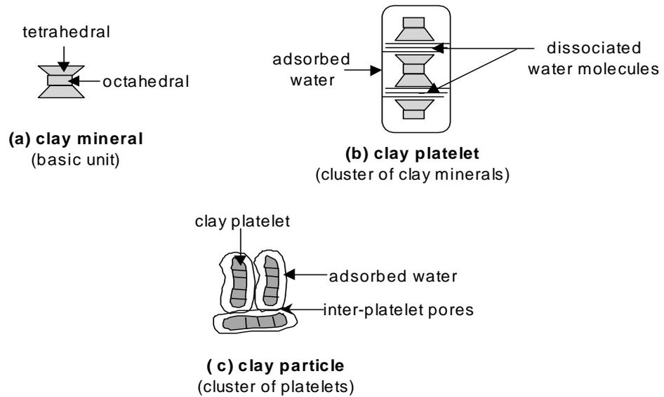
Figure 2.4 Illustration of the soil particle model
