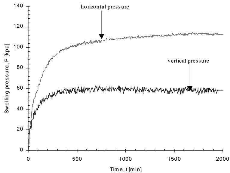
Figure 6.2 Mobilised swelling pressure for a sample compacted at LCE
