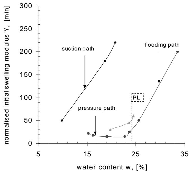
Figure 6.7 Swelling modulus - water content plot along atmospheric swelling
