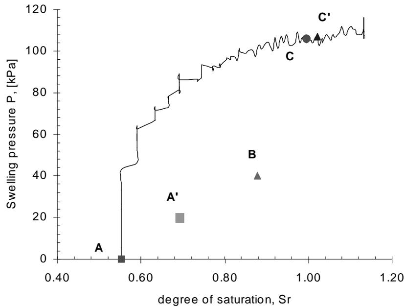
Figure 8.3 Degree of saturation - swelling pressure plot: pressure gradient wetting during confined swelling
