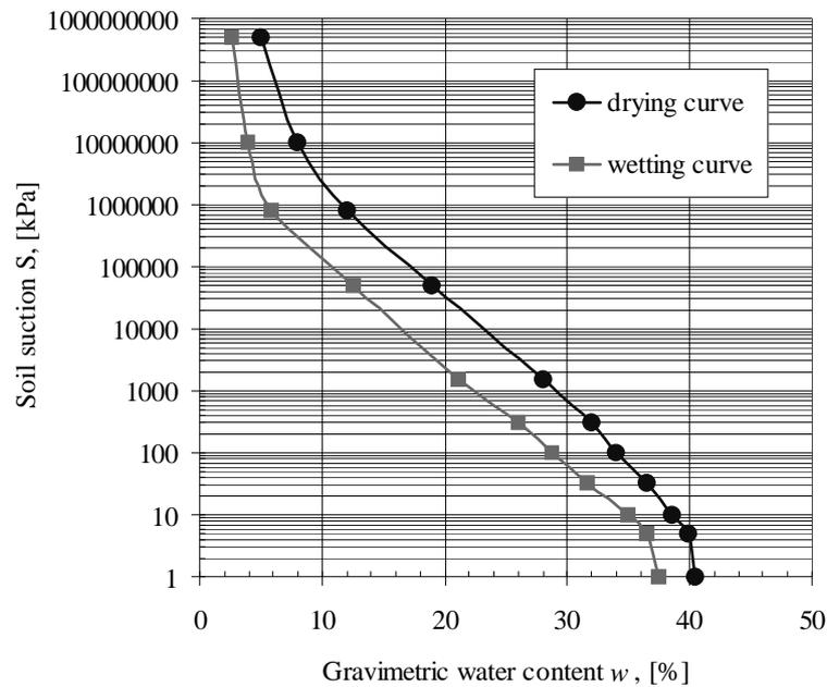
Figure 4.1 Soil-Water Characteristic Curve for Avon clay
