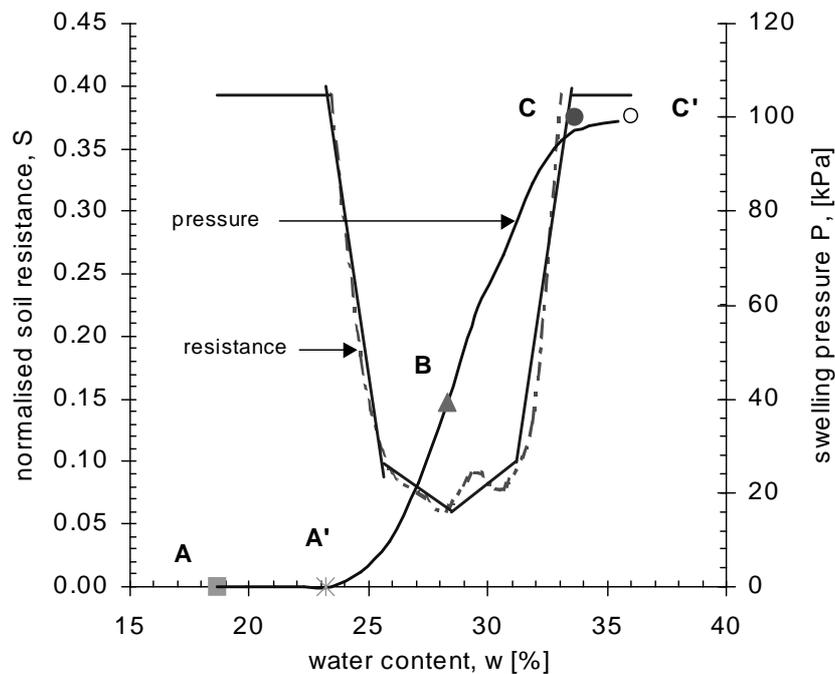
Figure 5.1 Soil resistance along suction-gradient wetting path
