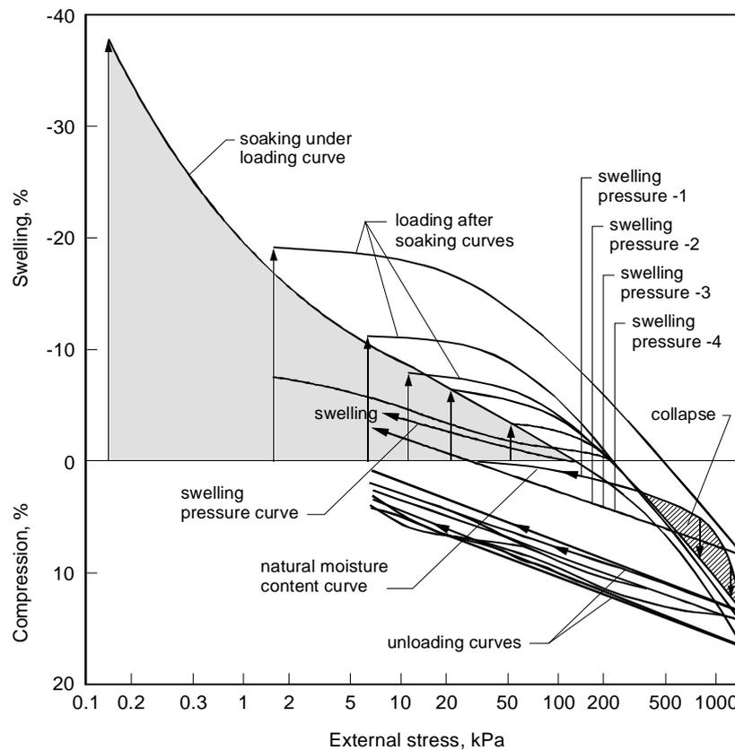
Figure 1.3 External stress - strain plot (after Justo *et al.* 1984)
