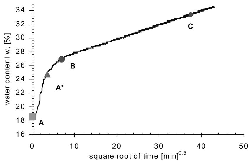
Figure 5.2 Increase of soil water content with time-suction gradient path
