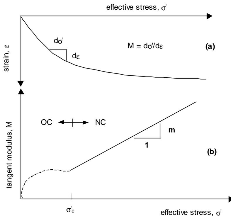
Figure 3.10 Stress-strain curve from an incremental oedometer test for clay.
