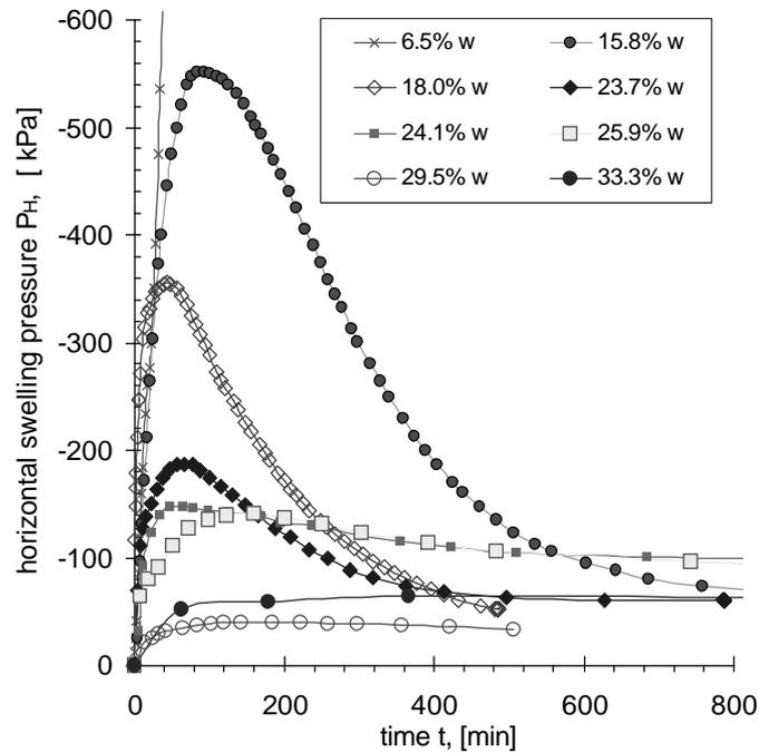
Figure 4.8 Swelling pressure - time plot (flooding path)
