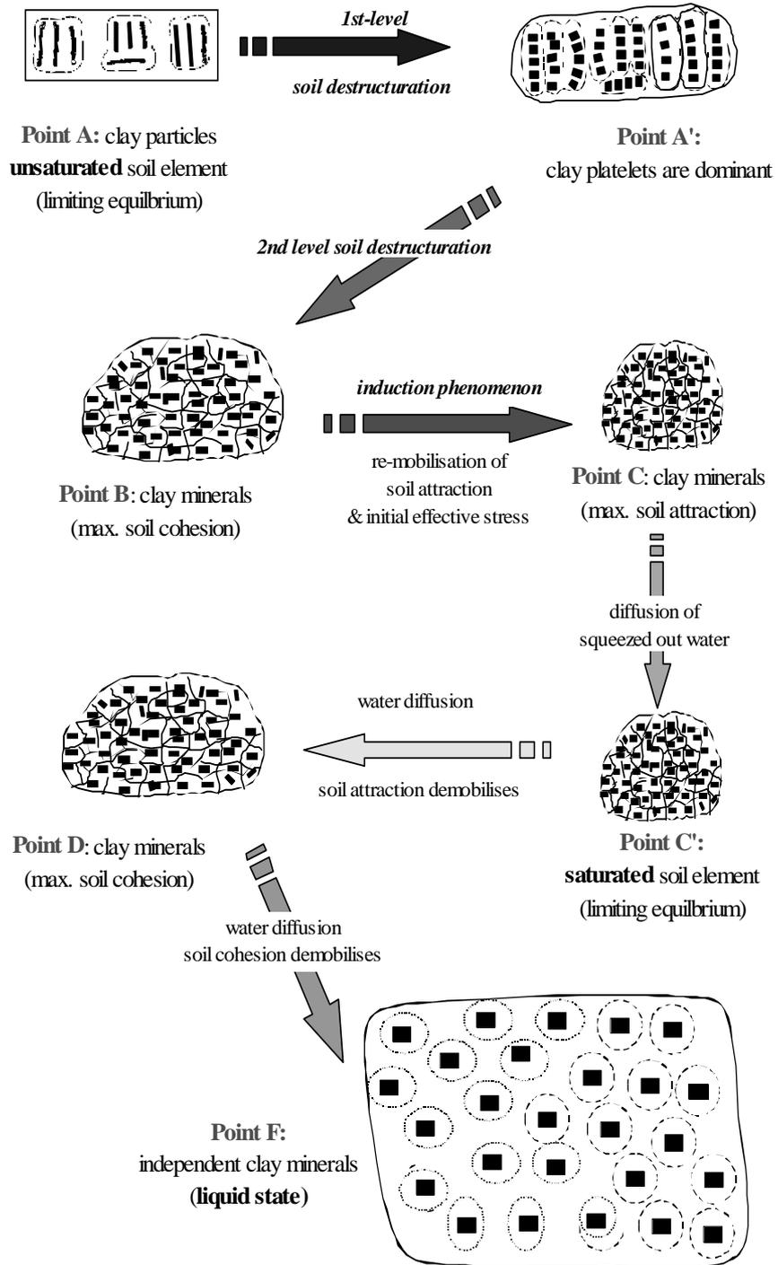
Figure 2.5 A model for the dynamic (changing) soil structure, featuring the deconstruction and induction phenomena.
