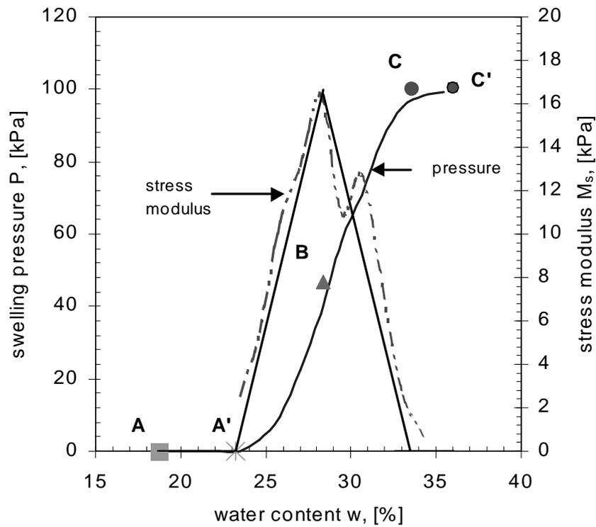
Figure 5.4 Swelling-pressure and stress resistance modulus curves
