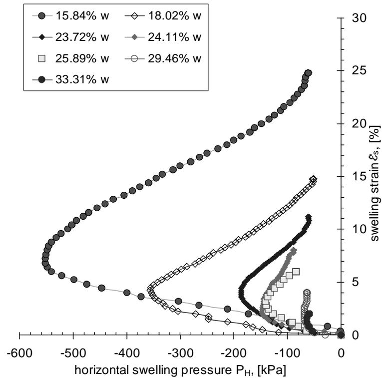
Figure 4.9 Swelling pressure - swelling strain plot (flooding)
