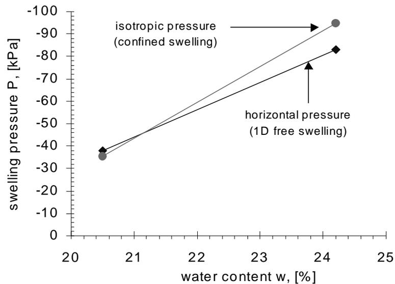
Figure 6.4 Comparison of swelling pressure measured during confined and unconfined suction-swelling
