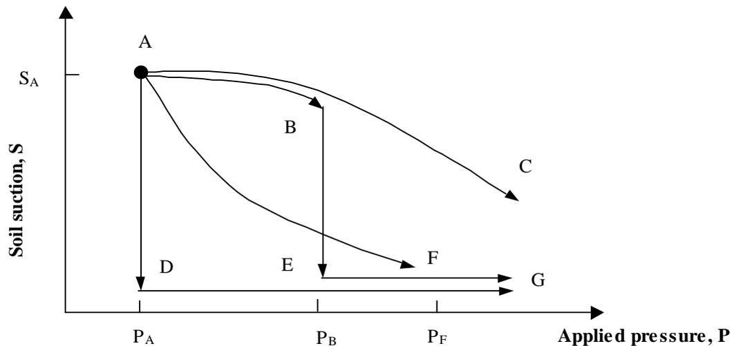
Figure 1.2 Typical stress paths in the  $(p, s)$  stress space (after Alonso *et al.* 1987)
