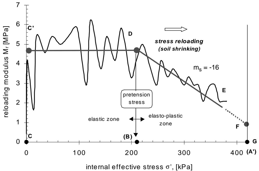
Figure 8.5 Reloading modulus plot. Initial water content = shrinkage limit
