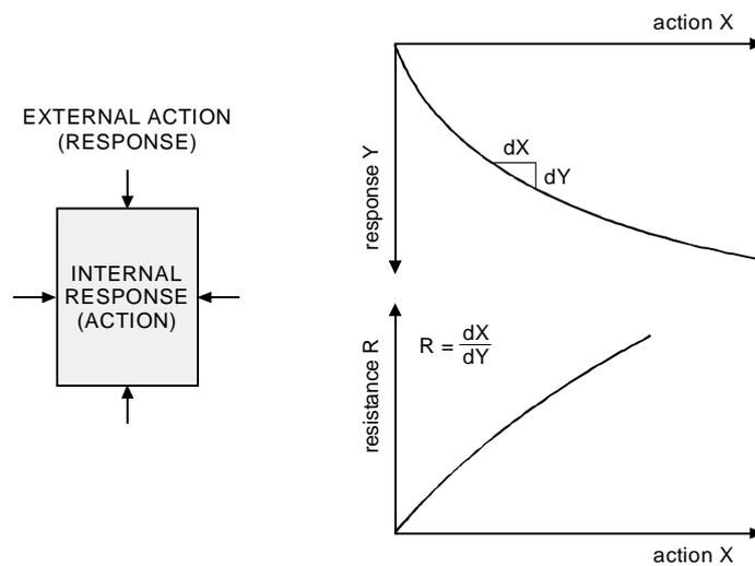
Figure 3.9 Definition of the resistance of a material (after Janbu, 1995, 1998)
