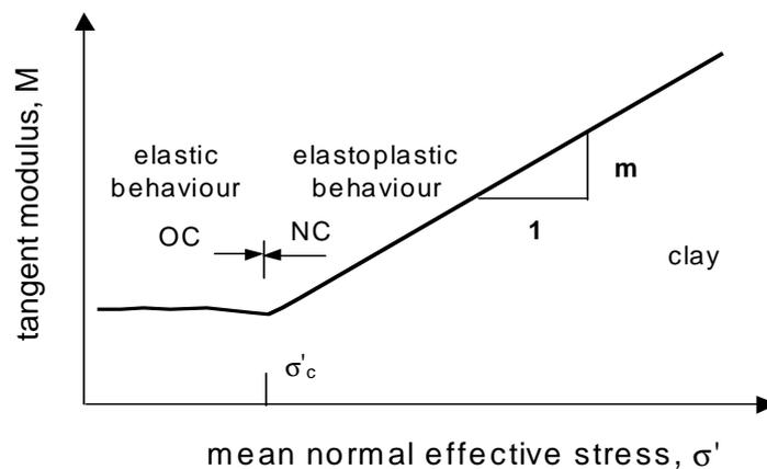
Figure 7.3 Idealised oedometer tangent modulus: over-consolidated soil (Janbu, 1963, 1998)
