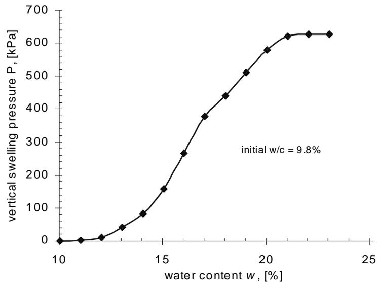
Figure 4.5 Water content - swelling pressure plot (suction gradient)
