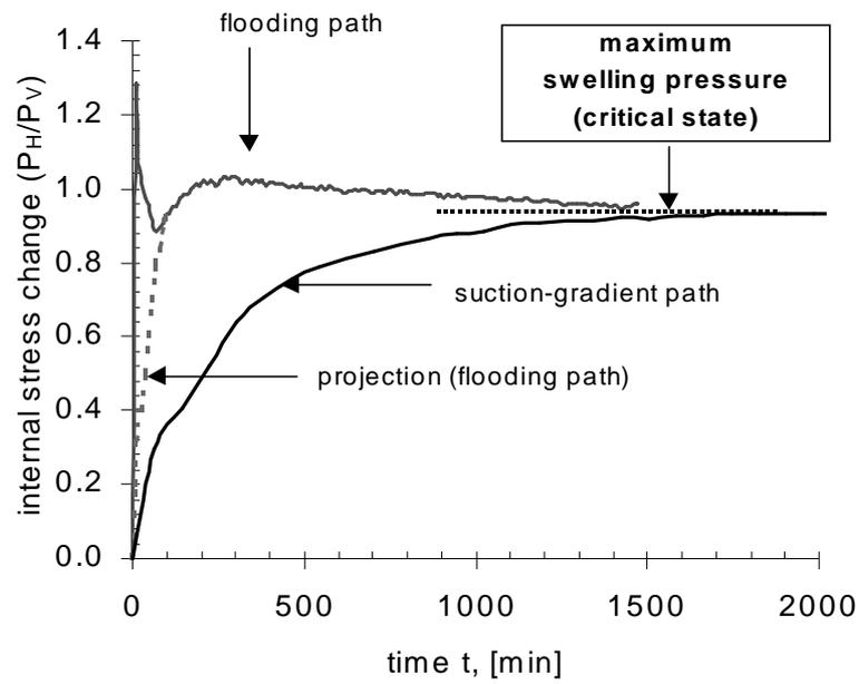
Figure 6.5 Change of the internal stress of the soil with time.
