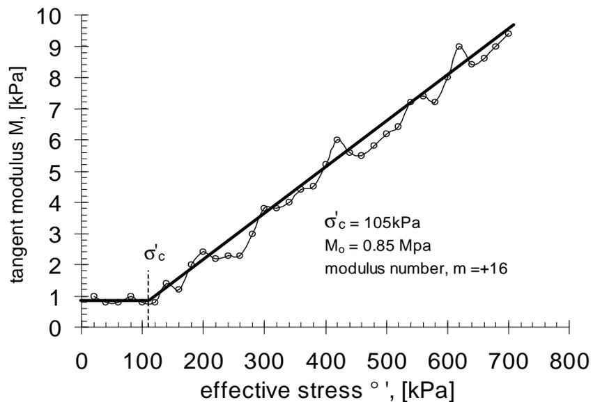
Figure 8.4 Consolidation test results on the investigated expansive soil.
