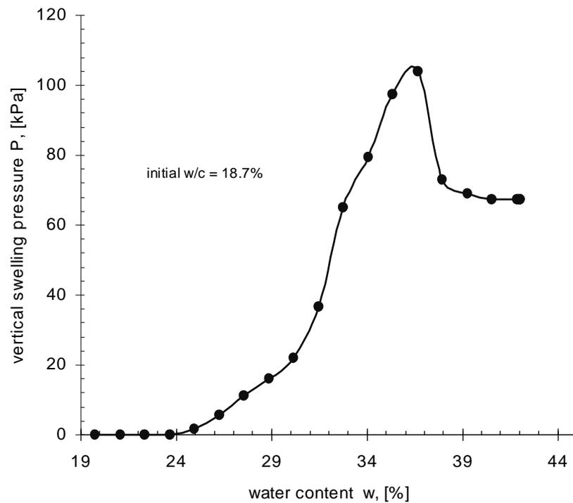
Figure 4.6 Water content - swelling pressure plot (pressure gradient)
