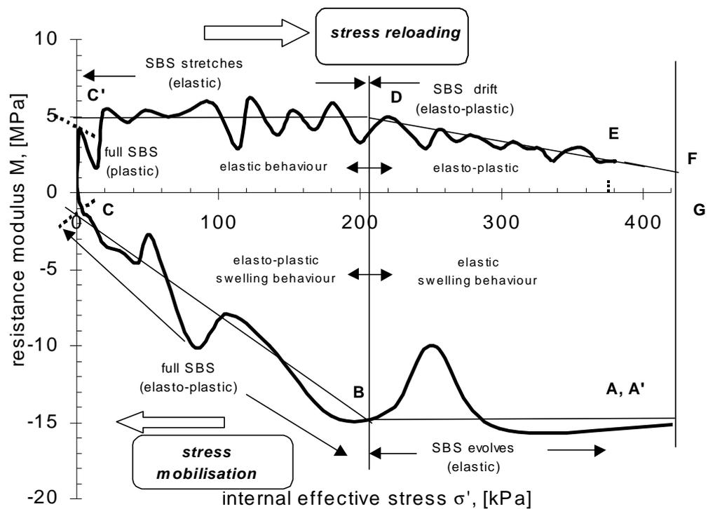
Figure 8.2 Internal effective stress-modulus plot at shrinkage limit
