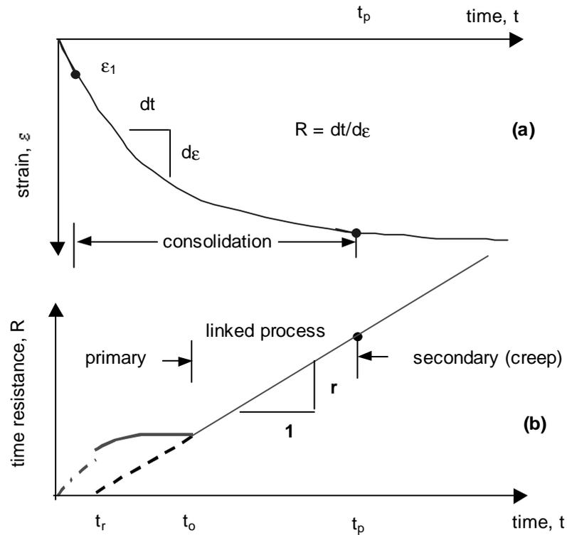
Figure 3.11 Time-strain curve of an incrementally loaded oedometer test
