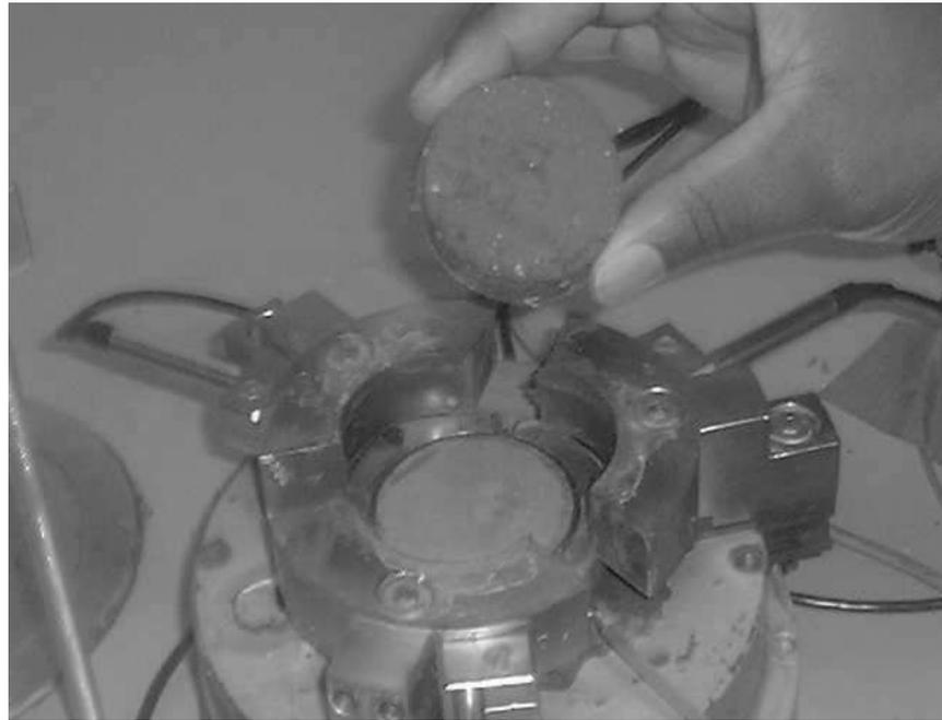
Figure 3.5 Placing of the soil sample in the split-ring oedometer
