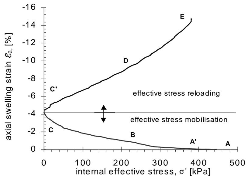
Figure 7.2 Stress-strain relationship along flooding wetting-path
