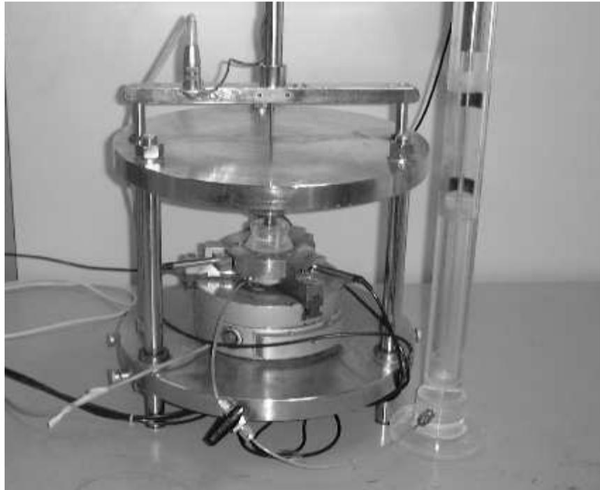
Figure 3.6 Oedometer set up for confined swelling tests
