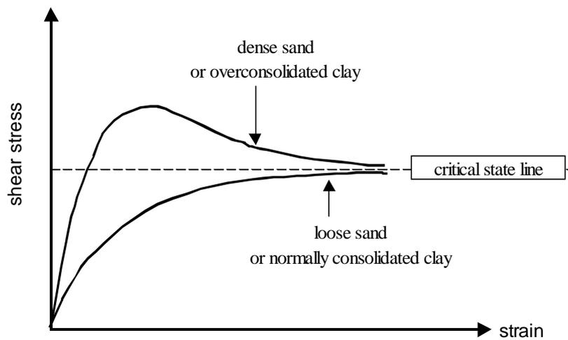
Figure 6.6 Illustration of undrained triaxial compression of saturated sands and clays.
