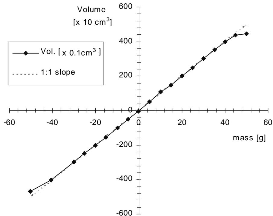
Figure 3.4 Calibration curve for the electronic burette
