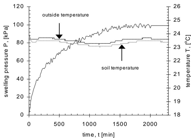
Figure 4.4 Change of soil temperature during confined soil swelling (suction gradient)
