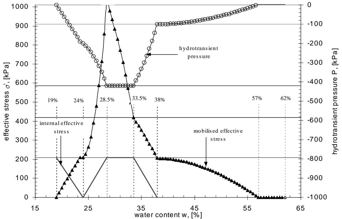
Figure 9.1 Coupling between the different forms of effective stress and water content
