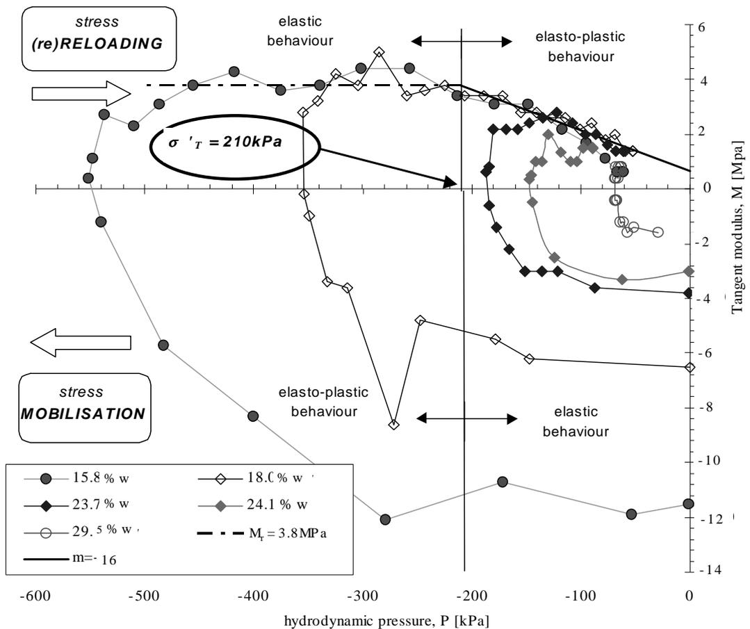
Figure 8.1 Determination of the pretension stress
