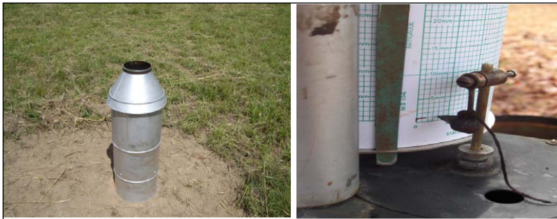
Figure 3.2 Autographic recorder under open sky (left) main frame (right) chart and recording pen.
