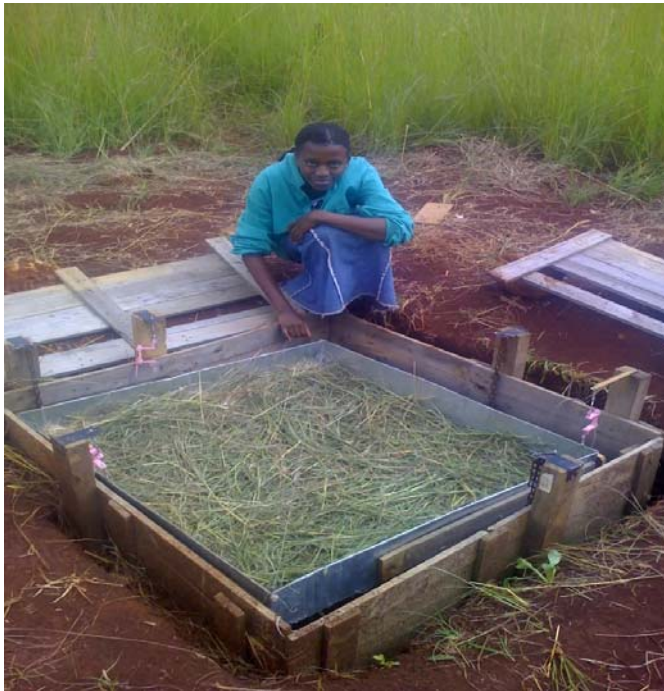
Figure 3.5 Setup of the forest floor interception device with upper basin containing Thatching ( Hyparrhenia filipendula ) grass
