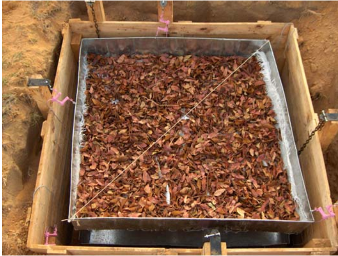
Figure 3.4 Setup of the forest floor interception device with upper basin containing Msasa ( brachystegia spiciformis ) leaf litter
