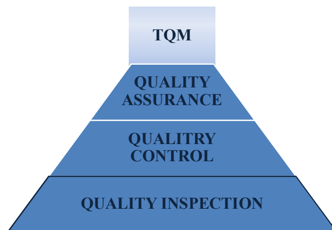
Figure 2.2: Pyramid 1 shows progression of quality from quality inspection, to quality control, quality assurance and lastly Total Quality Management (TQM).
