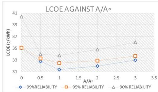
**Figure 6.** LCOE against A/A<sub>0</sub> for no generator with net metering
