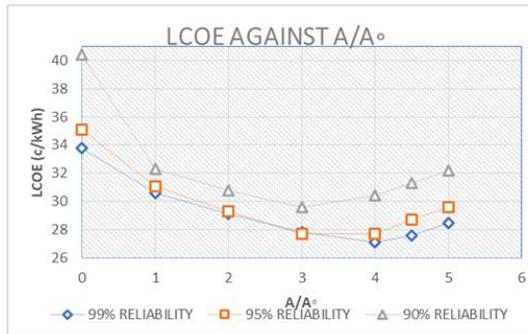
**Figure 7.** LCOE against A/A<sub>0</sub> for diesel generator yes and net metering yes
